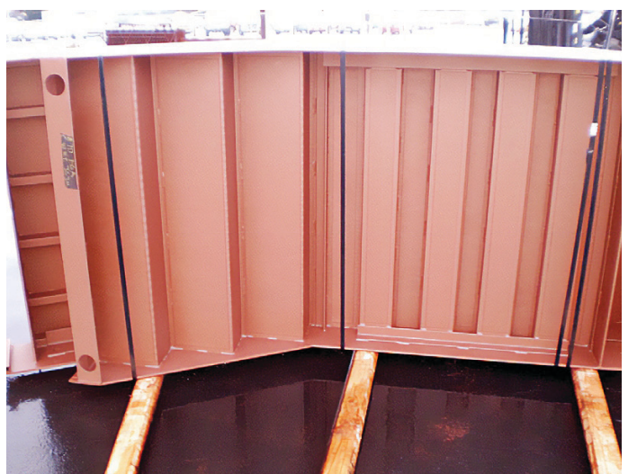
Painted with shop primer and ready for final color
