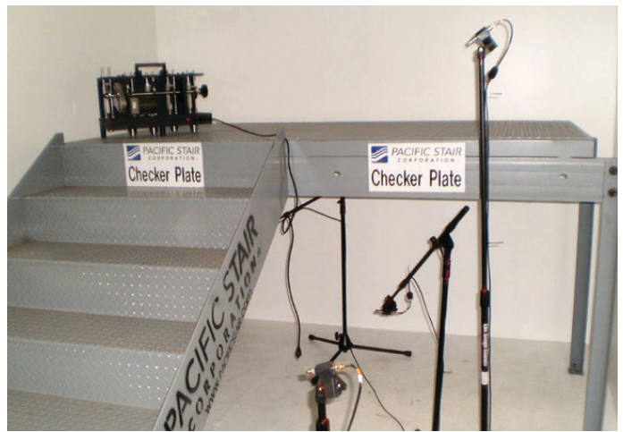
Landing only sound testing
