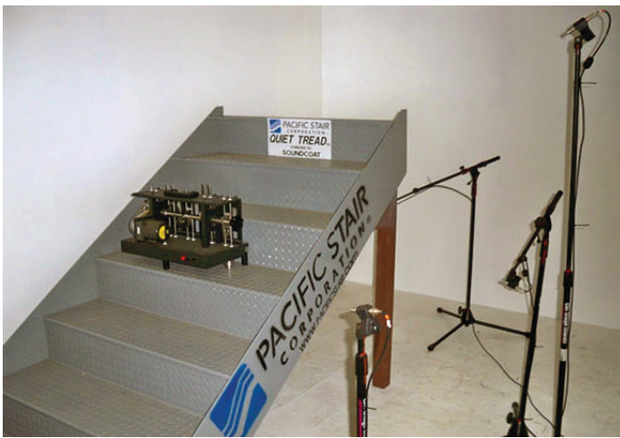
Stair only sound testing
